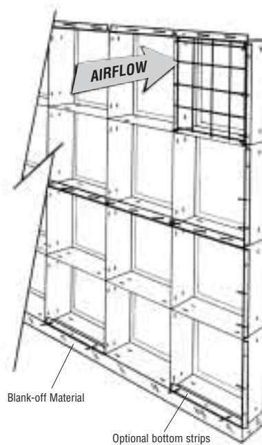
Columbus Industries' modular bank section (shown with roll conversion strips) makes conversions and new installations easy and economical.
